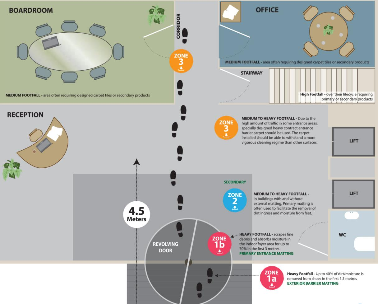
and 1b the installation of exterior matting catches the first wave of heavy debris in a high traffic area, ensuring the removal of up to 40% of dirt and moisture from entering the building. An effective primary entrance mat will continue the removal of dirt and moisture working with the external matting containing any heavy debris.
